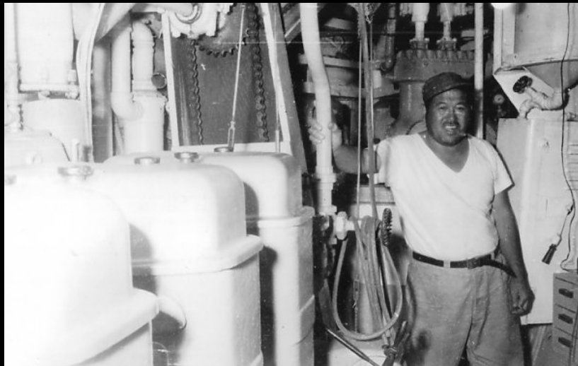
Richard Chikami's father, Min Chikami in the engine room of the Stella Maris in the 1950's. Min was the Chief Engineer and took care of the 400 Horsepower Enterprise main engine (left of picture).
