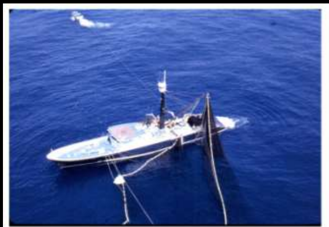
Step 1: A purse seine vessel initiating the back-down procedure with the skiff towing the vessel mid-ship to create the tear-drop net configuration needed to successfully depress the cork line and allow the dolphins to escape.
