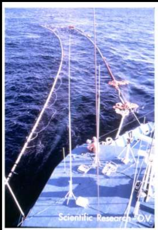
Step 3: The vessel "backing down" with main engine in reverse, submerging the cork line at the Medina Panel apex with dolphins being successfully released.
