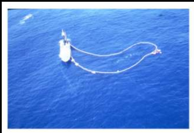
Step 2: The tear-drop net configuration as seen from the vessel's helicopter circling above. Note the speed boats positioned at the apex of the tear drop which corresponds to the location of the small mesh Medina Panel that facilitates the successful release of the dolphins.
